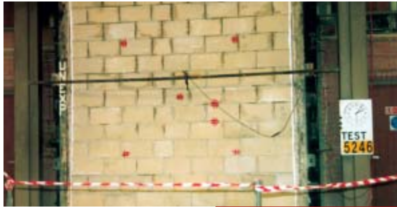
Fire test of reinforced wall
