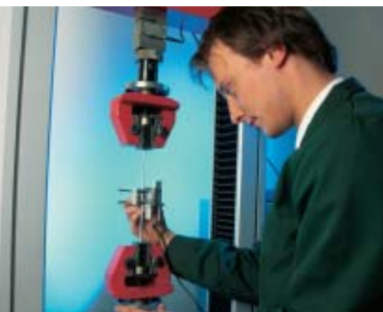
Daily testing of flattened wire
