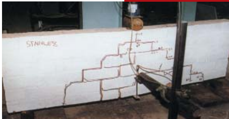
Test load being applied
