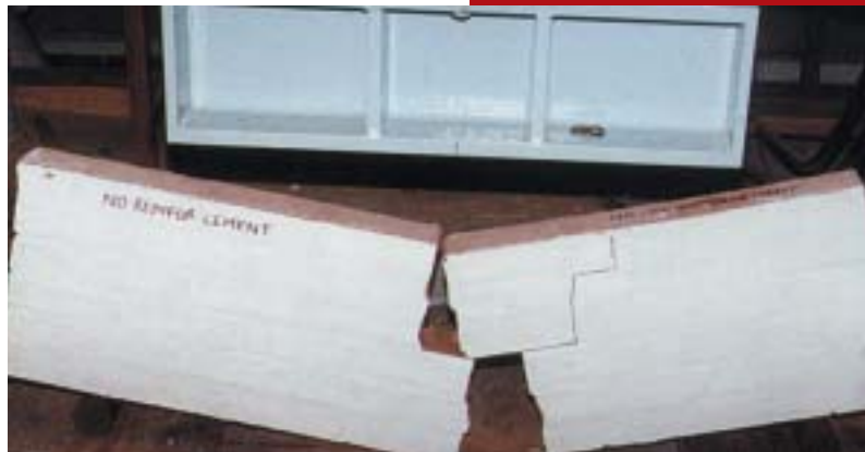
Failure of un-reinforced wall
